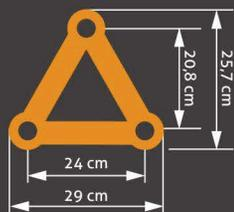
The weight of the truss is considered in the load table.
